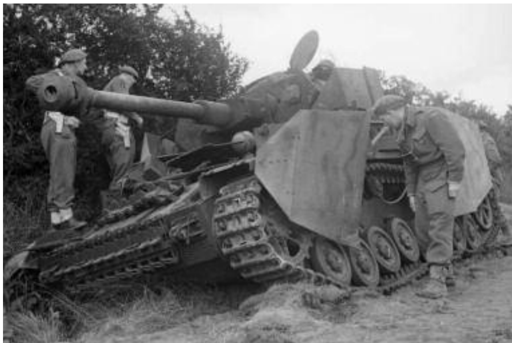
Officers inspect a German Mk IV tank knocked out by the Durham Light Infantry - 11 June 1944. The tank is equipped with Schürzen ("aprons"), armoured plates adopted during the Russian campaign to protect the tanks against Soviet AT rifles. In due time Schürzen became also useful to pre-detonate HEAT bazooka warheads. Copyright © IWM (B5375)
